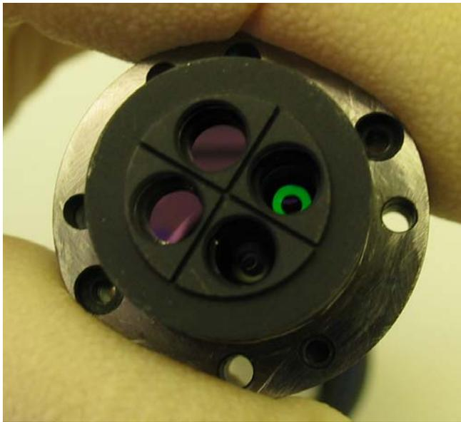
Figure 7 Rear View of VMC Optics (green: VIS, purple: NIR channels)
