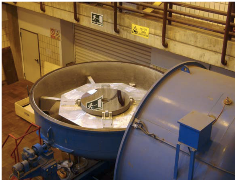
Figure 4. SolarLite mirror after Al-coating mounted in the IAC coating chamber.
