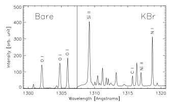
**Fig. 2.** Examples of analysed SUMER spectra. The upper two frames were recorded mainly on the potassium bromide (KBr) photocathode (within the two vertical lines) while the lowest frame shows a spectrum partially recorded on the bare microchannel plate and partially on KBr (separated by the vertical line). The spectra are averaged over the slit length. The analysed lines are identified.
