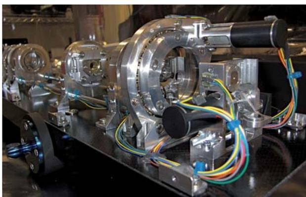
**Fig. 3** (online colour at: [www.an-journal.org](http://www.an-journal.org)) Wave-front sensor of SUNRISE. The picture shows, from right to left, the (motorized) focal plane unit of the CWS, the (motorized) neutral density wheel and the mount for the micro-lens array, together with some re-imaging lenses.
