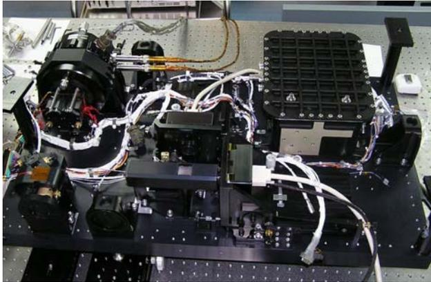
**Fig. 4** (online colour at: [www.an-journal.org](http://www.an-journal.org)) IMaX spectropolarimeter during assembly in Madrid. The LiNb etalon is in the upper left corner of the picture. The two CCD detectors are at the center (facing left and down), and the box on the upper right contains the electronics for the etalon.
