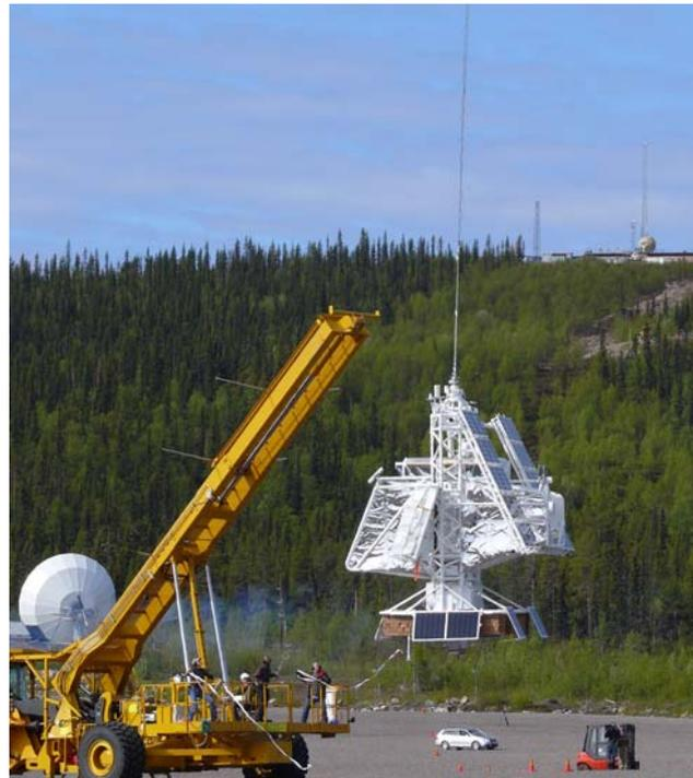
**Fig. 5** (online colour at: [www.an-journal.org](http://www.an-journal.org)) Launch of Sunrise at ESRANGE in the morning of 8 June 2009. The gondola with the telescope stowed in horizontal position has just been released from the launch vehicle. The solar panels for the science payload are mounted on both sides of the telescope. The small solar panels below the telescope are used for the telemetry system.
