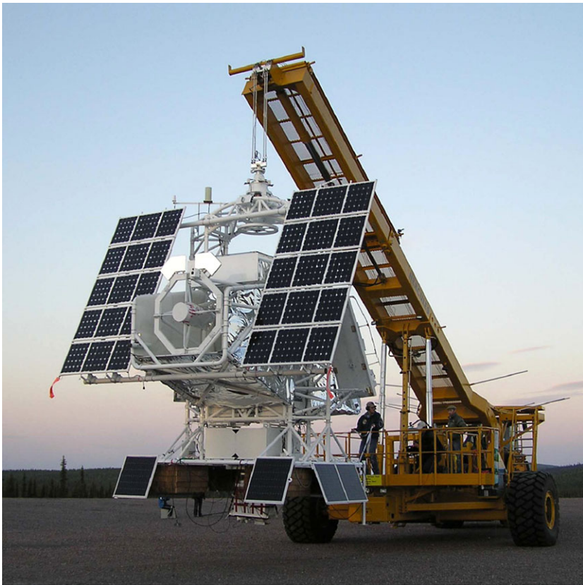
Figure 1 Overview of the Sunrise observatory in full flight configuration, immediately before launch. The dimensions of the observatory can be judged by comparing with the person on the launch vehicle. In the center of the gondola the telescope front ring can be seen, with the radiators for the heat rejecting prime focus field stop. The box on top of the telescope is the postfocus instrumentation (PFI) platform housing the science instruments. A flywheel below the upper bridge of the gondola structure is used for azimuth pointing. Instrument electronics is mounted on two inclined racks on the rear side of the gondola. The white box in the lower part of the gondola is the CSBF-provided system instrumentation package (SIP), needed for commanding of balloon and payload. It uses a dedicated power system, while the main power for the observatory is generated by the large solar arrays to both sides of the telescope.
