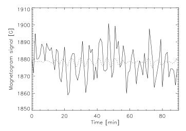
**Fig. 5.** The solid line is the same as in Fig. 2a. The dotted line represents the magnetogram signal that would be expected from cross-talk from the velocity oscillations.
