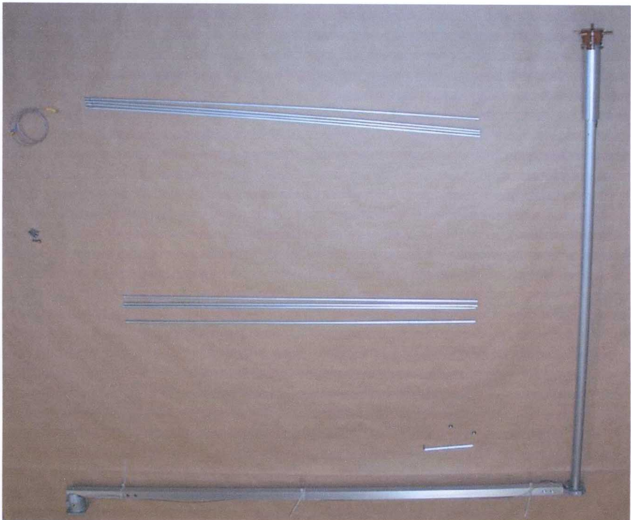
Fig. 2: Dipole head, vertical and horizontal masts and cable assembled
