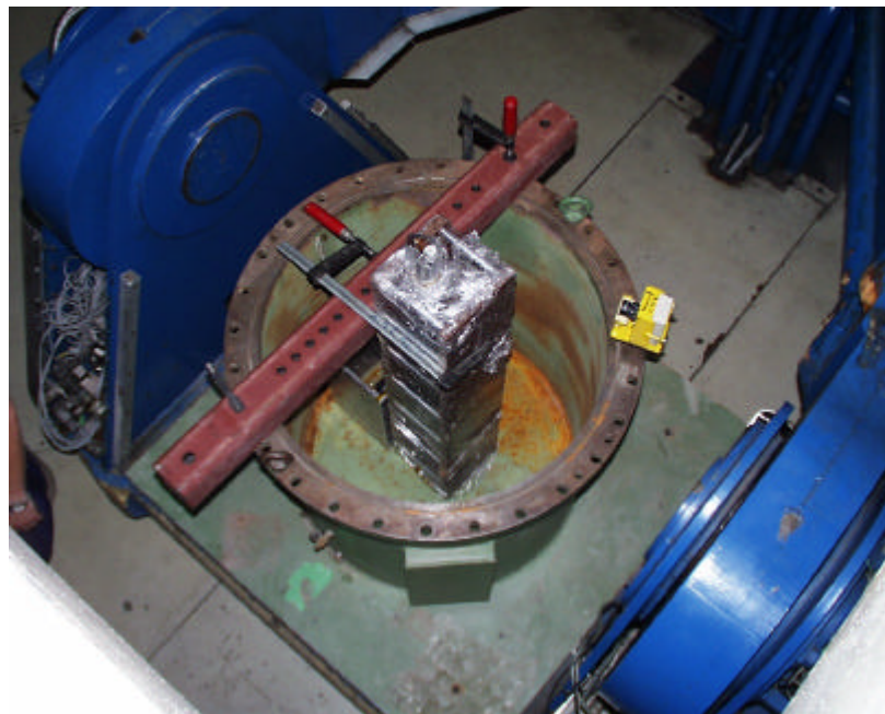
Mounting Antenna and E-Box on Centrifuge-Platform for +X-Axis
