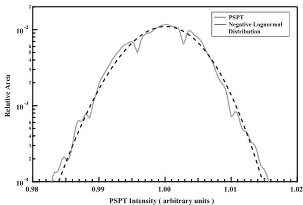
**Fig. 5.** Intensity histogram of the broadband image obtained at the Mauna Loa Observatory on 2005, Feb. 26 at around 6060 Å compared with a single modified log-normal distribution function. The wiggles are an artifact of digitization and were smoothed.
