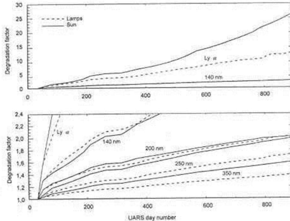
Optical path degradation of SUSIM during 2.5 years of the UARS mission
