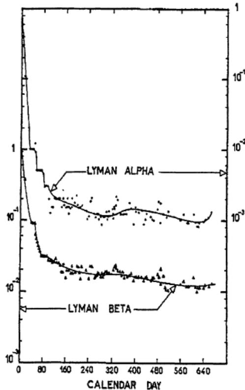
Figure 6 — Variations of the sensitivity of the LPSP instrument on OSO-8. The ordinate gives the value relative to that at launch, and time on the abscissa is given in days after launch.
