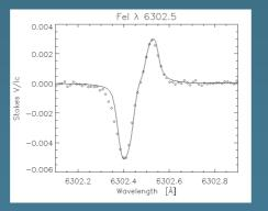
2 magnetic structures provide a reasonable fit for both Stokes V Profiles But these structures have a finite correlation ! Correlation lengths between 50 km and 125 km Filling factors are 2.7% and 2.1%
