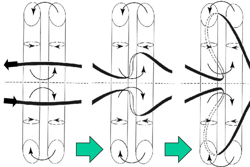
Advection and twisting of toroidal field lines (assuming frozen flux) by helical columnar flow, transforming them into configuration with strong poloidal dipole part
