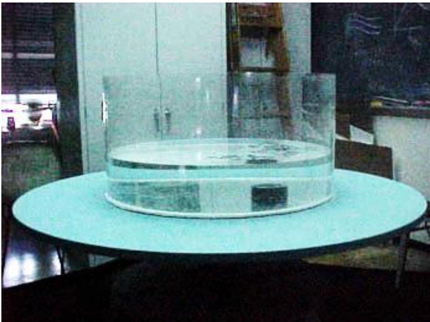
Cylindrical water tank on rotating table with small off-center obstacle on bottom
