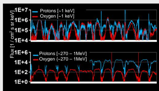
The figure to the right shows one month of Cluster proton and oxygen data for two energy ranges. During some times, and for some regions of space, the flux of oxygen exceeds that of protons.
