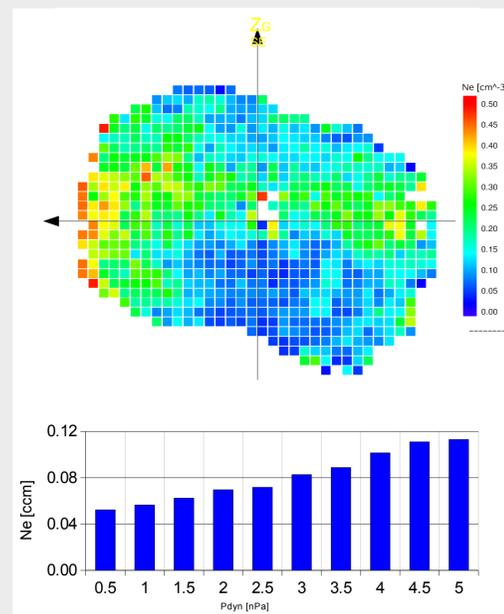
The low plasma density combined with strong spacecraft charging usually makes direct measurements difficult in the magnetotail lobes. However, a new technique makes use of the spacecraft potential to derive information about electron density.
