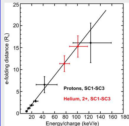
The RAPID detector has been used to determine field aligned density gradients at the terrestrial bowshock. Our results show that the diffuse ions are subject to diffusive transport and that the ion partial densities decrease exponentially with increasing distance from the bow shock.
