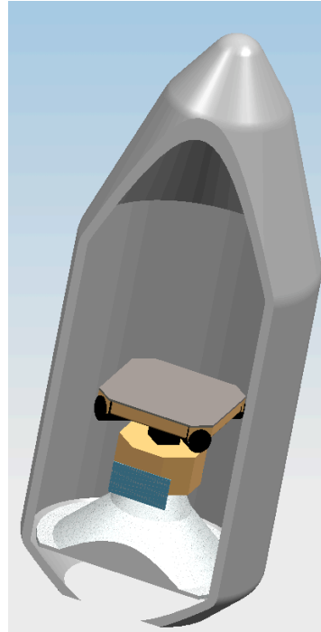
Figure 14: View of the spacecraft with the solar sail in launch configuration in the 4-m diameter Soyuz fairing. Spacecraft dimensions are derived from [RD2] (View courtesy of J.-C.Leclec'h).
