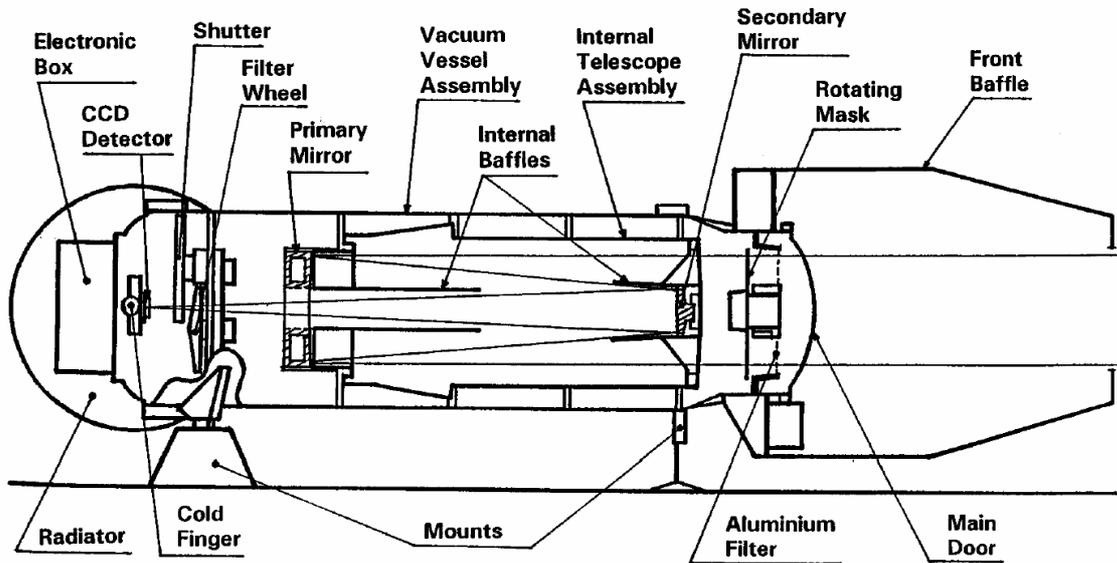
Figure 2.5. Schematic view of the EIT instrument and its main components. Adapted from Delaboudinière et al. (1995).
