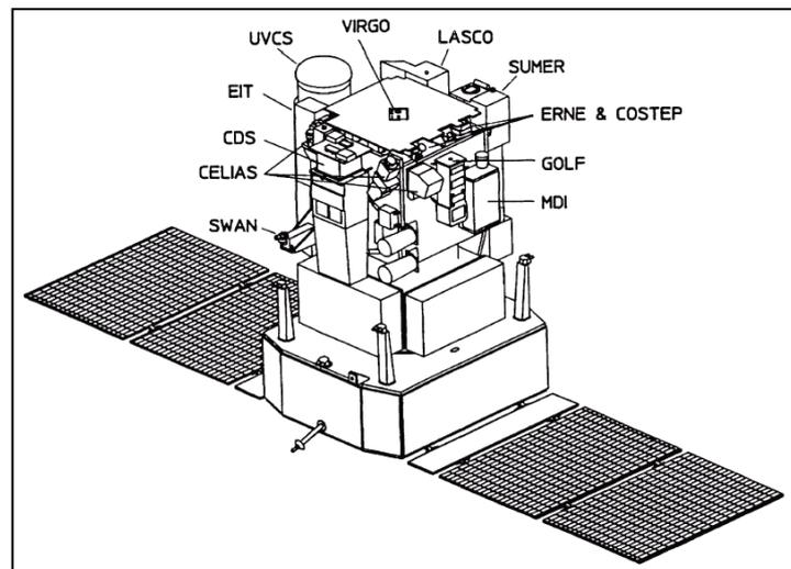
Figure 2.2. Schematic of the SOHO spacecraft and its payload. Adapted from Domingo et al. (1995).
