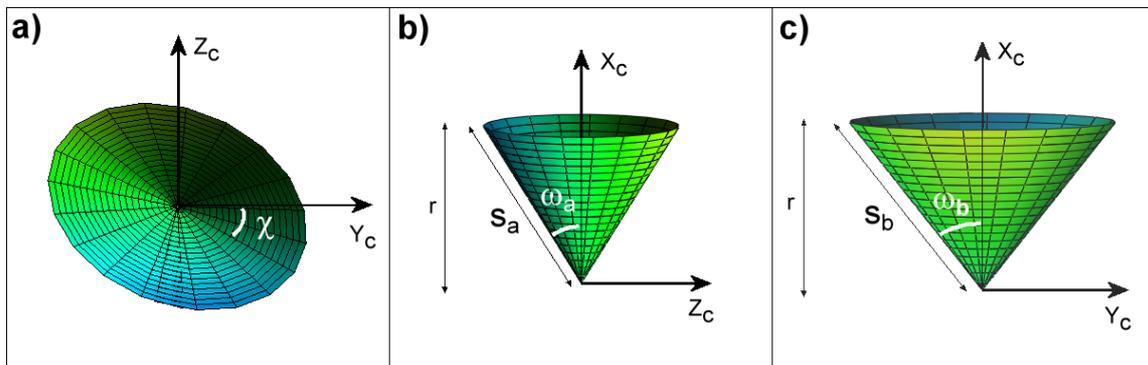
Figure 4.3. Three views of an elliptical cone generated by the elliptical cone model with width  $\omega_a=30^\circ$  and  $\omega_b=40^\circ$ . a) Plane  $Z_cY_c$ : the base of the cone, with  $\chi=20^\circ$ . b) Plane  $X_cZ_c$ : minor width  $\omega_a$  of the cone. c) Plane  $X_cY_c$ : major width  $\omega_b$  of the cone.
