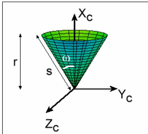
Figure 4.1. A circular cone in its coordinate system. The axis  $X_c$  is aligned with the central axis of the cone, and the axes  $Y_c$  and  $Z_c$  are orthogonal. The half AW of the cone is given by  $\omega$ , while  $r$  and  $s$  are the radial distance and the slant height respectively.
