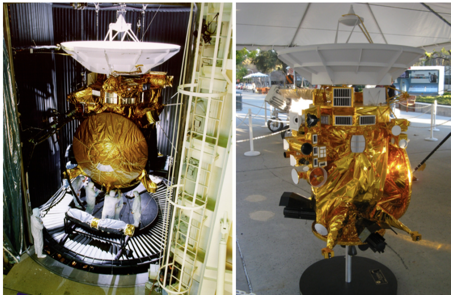
Figure 3.1: Cassini with Huygens probe. Left hand side: picture of the spacecraft before launch, see engineers for size comparison. Image courtesy of NASA/JPL/SSI. Right hand side: model of the Cassini spacecraft at JPL, January 2008.
