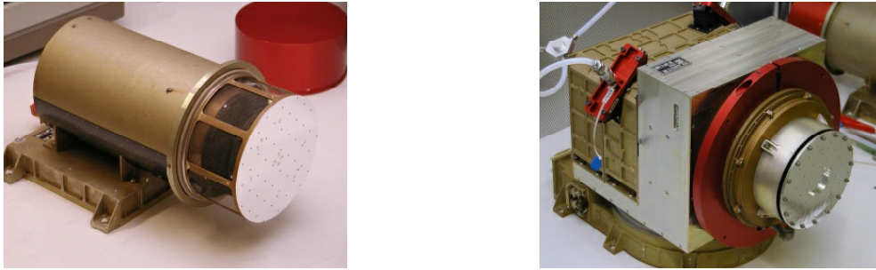
Figure 2.2: The IMA sensor (left) and the Main Unit with the ELS in view (right)
