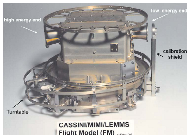
Figure 2.7: A flight test model of the LEMMS sensor, with its main parts indicated.
