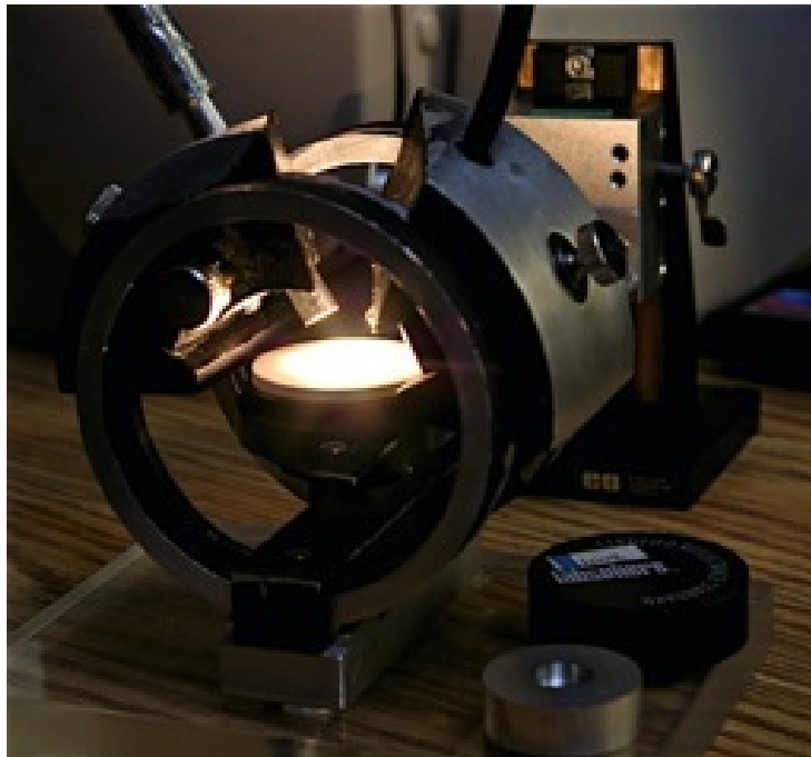
Figure 4.8: Goniometer used to acquire laboratory spectra at the University of Winnipeg Planetary Spectrophotometer Facility. Reproduced from http://psf.uwinnipeg.ca/Facilities.html .
