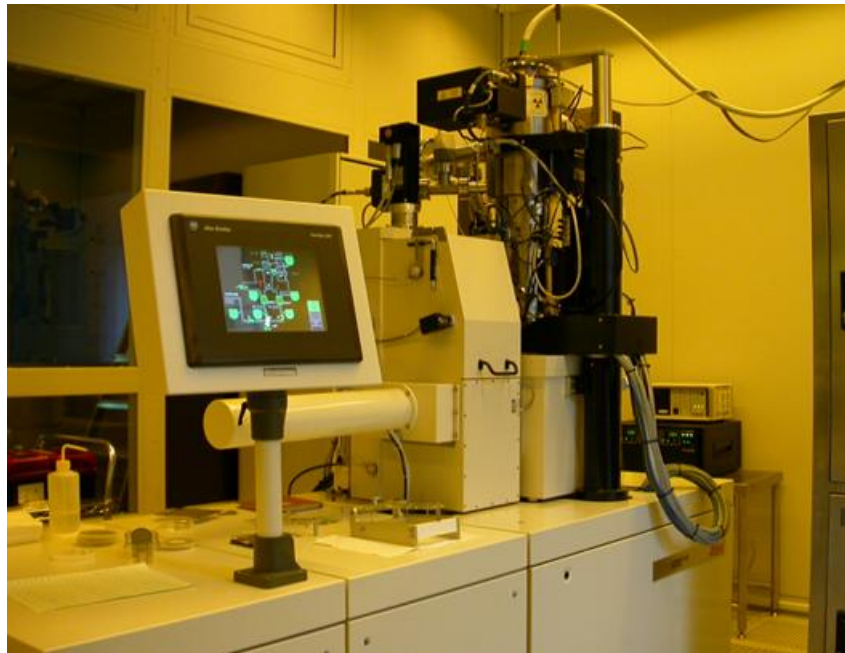
Figure C.1: Photo of the EBPG5000+ e-beam lithography system in the clean room center of PTB.
