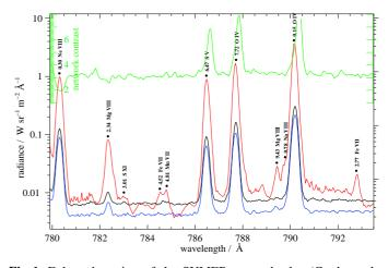
**Fig. 1.** Enlarged portion of the SUMER spectral atlas (Curdt et al., 2001) showing radiances of average QS (black), sunspot (red), and coronal hole (blue) regions. The network contrast (ratio bright network/cell interior in green), which is normally around 3, increases to values of 6 to 8 in TR lines, and the centroids of the contrast profiles are clearly redshifted.
