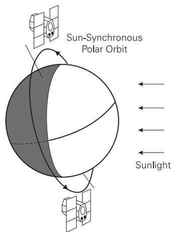
**Fig. 1.** Spacecraft observing from a Sun-synchronous polar orbit
