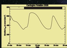
Fig. 4: Simulated solar wind velocity and magnetic field polarity at Machholz (black and white bar) following MHD modelling [3]. Changes in polarity cause ion tail disconnections. On 20.1, the velocity was expected to be changing fairly rapidly, from around 320 to >600 km/s in less than a day.
