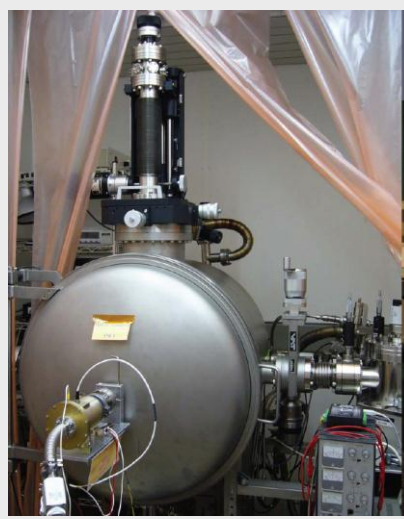
Photocathode deposition chamber and VUV vacuum test chamber
