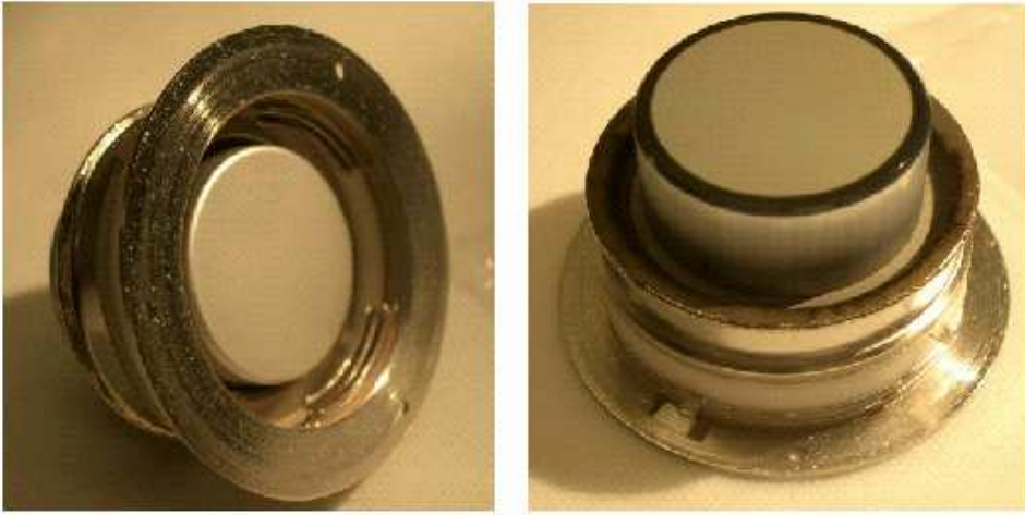
Figure 25.3: Intensifier housing with fibre optic output window. Left: inside-view with the phosphor screen and the pads for placing the 25 mm circular MCPs. Right: the fibre-optic output window at the back side of the tube.
