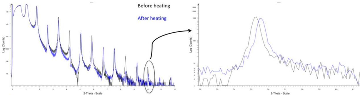
Figure 3-1: XRR measurement of a thermal test sample. The shift in the peaks enlarged on the right panel correspond to a multilayer period thickness change of 0.043 ( $\pm 0,003$ ) nm.
