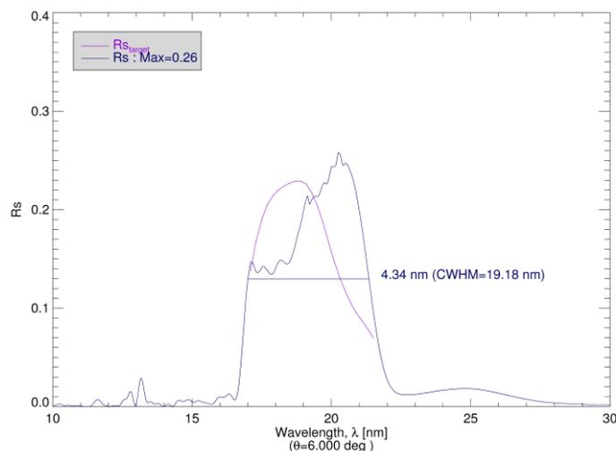
Figure 3-4: Stochastic design with higher emphasis on reflectance in the 19 to 21 nm range. The target specification is also shown.
