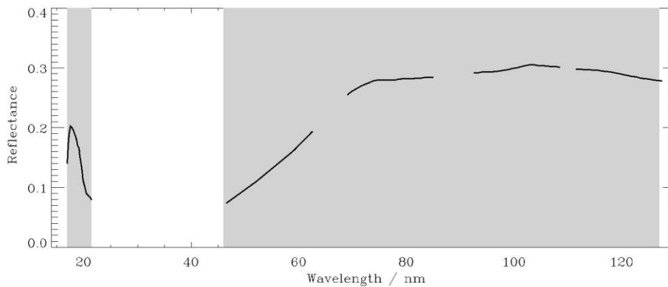
Figure 2-1: Target reflectance in the selected spectral regions (from data used by [4] and computed by combining literature values and experimental data).
