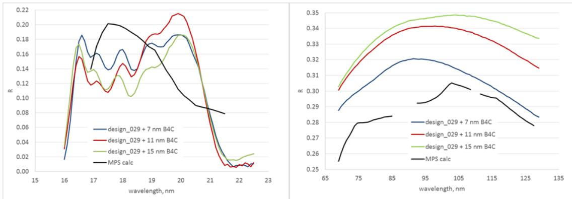
Figure 4-1: Measured reflectance in the EUV and VUV range for 7 nm, 11 nm and 15 nm of B<sub>4</sub>C on top of multilayer structure.
