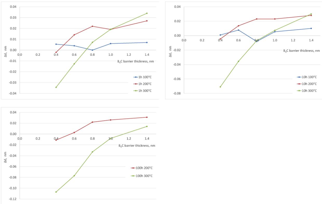
Figure 3-2: Change in period layer thickness depending on  $B_4C$  interdiffusion barrier thickness, temperature and test duration.
