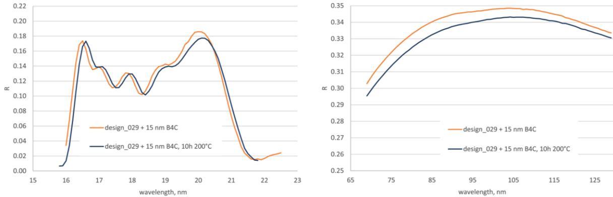
Figure 4-3: EUV and VUV reflectance before and after testing the final broadband coating for 10 h at 200°C.
