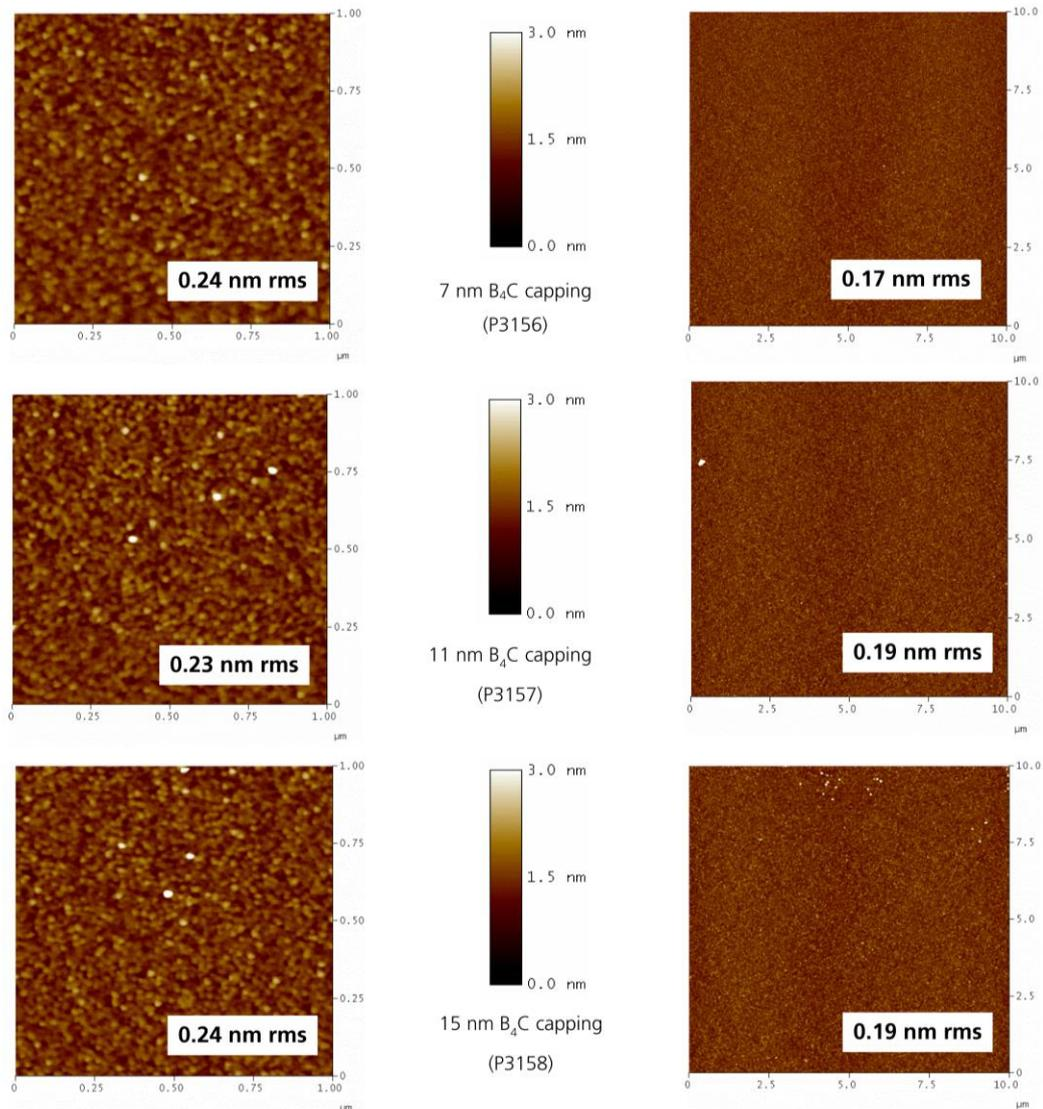
Figure 4-2: Roughness of multilayer coating with different B<sub>4</sub>C cap layer thicknesses.
