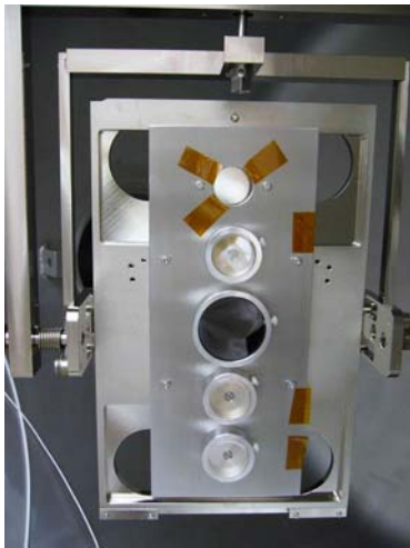
Figure 1: The sample holder inside the reflectometer with one blank quartz plate, three quartz samples coated with thin SiC (transparent) and the solid SiC/CVD reference sample (black) in the centre of the sample holder. A manipulator allows sample movements with five degrees of freedom. A detector can be rotated independently around the centre of the chamber.
