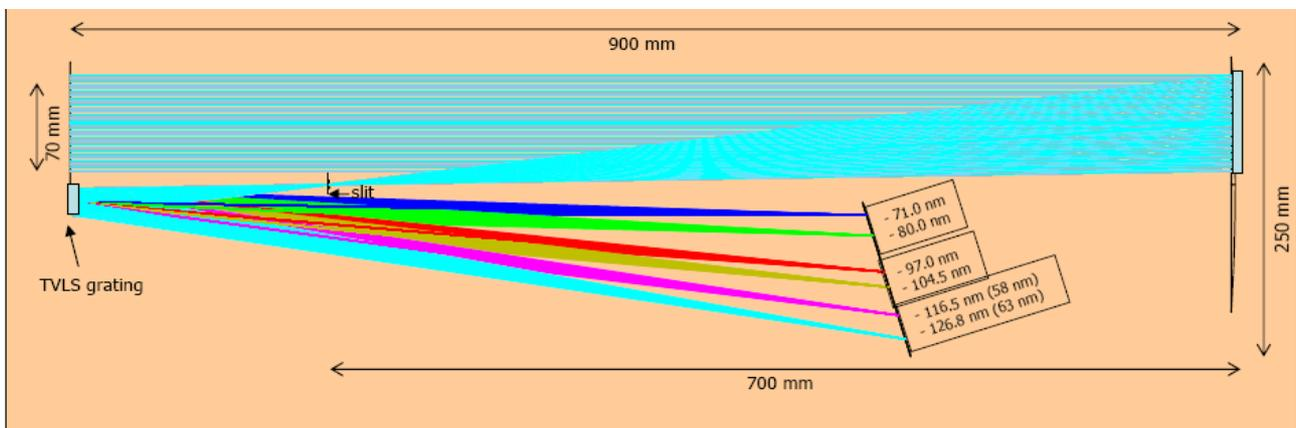
Figure 3: Optical design of a possible Extreme Ultraviolet Spectrometer (EUS) with three wavelength ranges between 71 nm and 127 nm.
