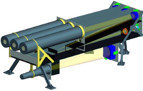
Figure 2: A possible design of the Extreme Ultraviolet Imager (EUI) suite of telescopes, consisting of three high-resolution imagers and one Full Sun Imager (courtesy of F. Auchere, IAS).
