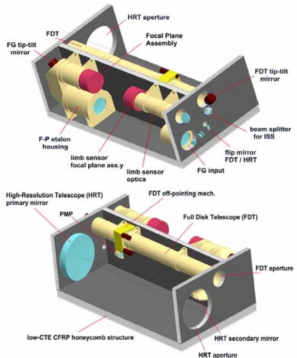
Figure 1: Sketch of the possible layout of the Visible-light Imager and Magnetograph (*VIM*) instrument (courtesy of H. Hartwig, MPS).
