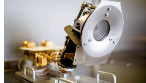
Solar Probe Cup (SPC)
