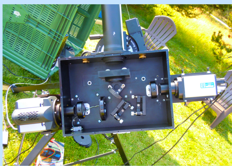
View of the SECIS II system with beam splitter, filters, lenses and 2 CCD cameras.
