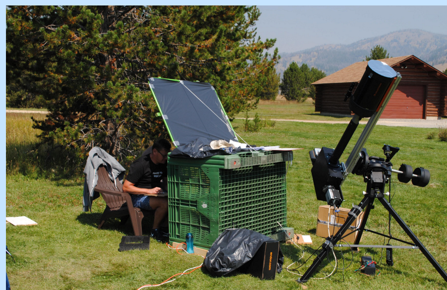
Observing setup: 20 cm telescope, SECIS II system with 2 cameras for the white light and 530.3 nm coronal line
