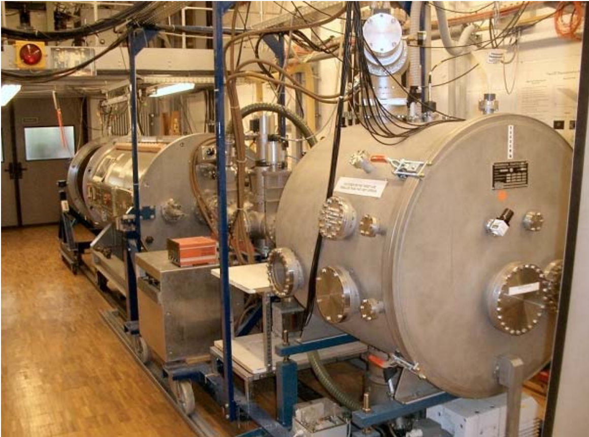
CASSINI Test Chamber designed to accommodate the engineering model of CDA
