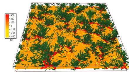
Figure 1: 3D visualization of vortex features (green) emerging from strong magnetic regions
