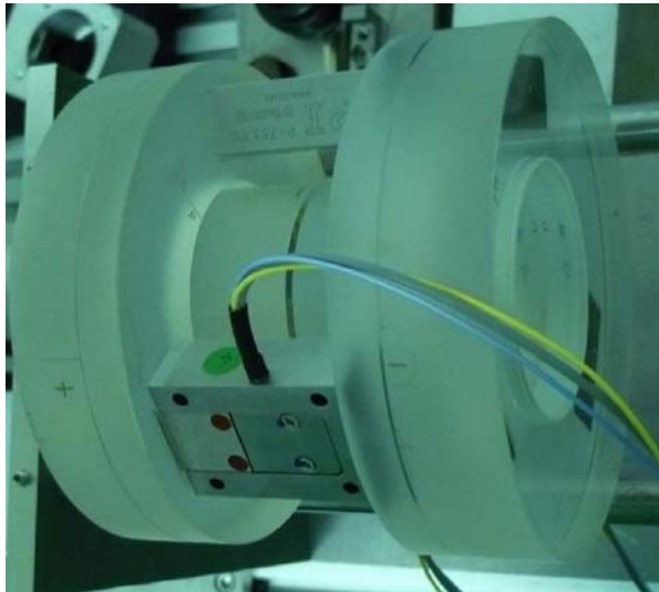
Fig. 5 Fabry–Perot etalon developed by Winlight, France as a prototype for SolO [32]
