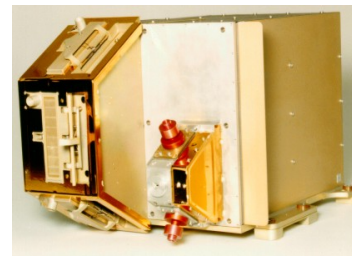
Fig. 9: The RAPID experiment with the ion (left) and electron (right) spectrometers.
