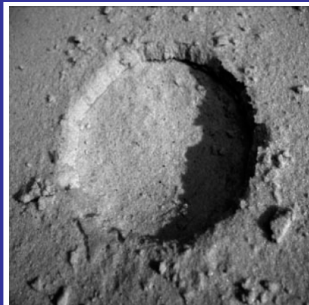
Fig. 5. A 10-cm-sized laboratory hypervelocity impact crater made as an analog of Wild 2's flat-floor craters. The crater was made with a 3.2-mm ceramic projectile impacting a porous target at 2 \text{ km s}^{-1} .
