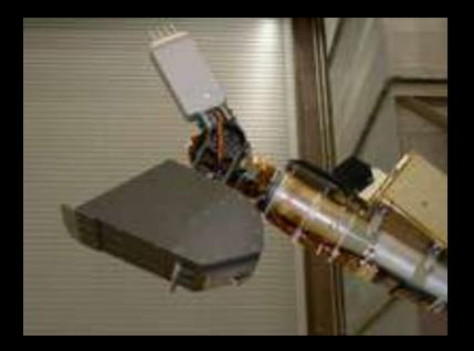
Thermal and Electrical Conductivity Probe (TECP)
