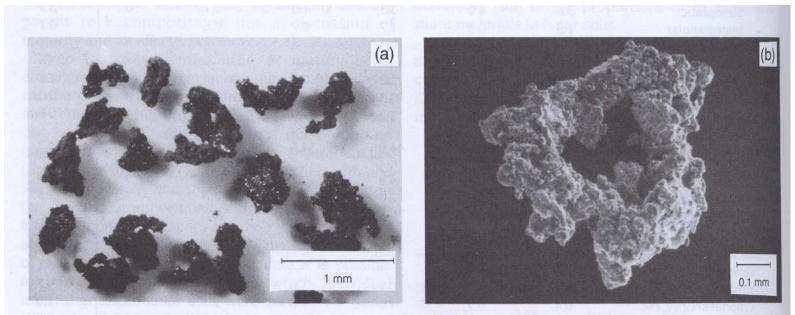
**Fig. 7.2.** Typical lunar soil agglutinates. **(a)** Optical microscope photograph of a number of agglutinates separated from Apollo 11 soil sample 10084, showing a variety of irregular agglutinate shapes (NASA Photo S69-54827). **(b)** Scanning electron photomicrograph of a doughnut-shaped agglutinate. This agglutinate, removed from soil 10084, has a glassy surface that is extensively coated with small soil fragments. A few larger vesicles are also visible (NASA Photo S87-38812).
