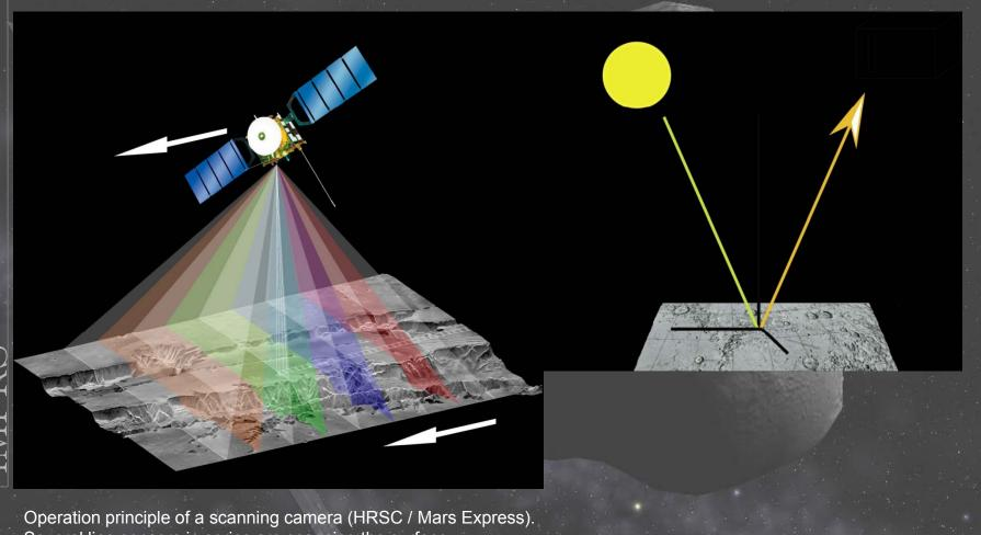
Several line sensors in series are scanning the surface.
