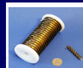
Figure 1: Drift tubes of different size: conventional (left), miniaturized (right)
