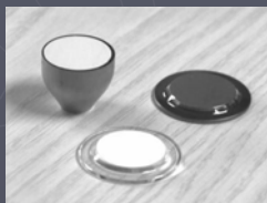
Phosphor screen anode on fiber optic coupler
