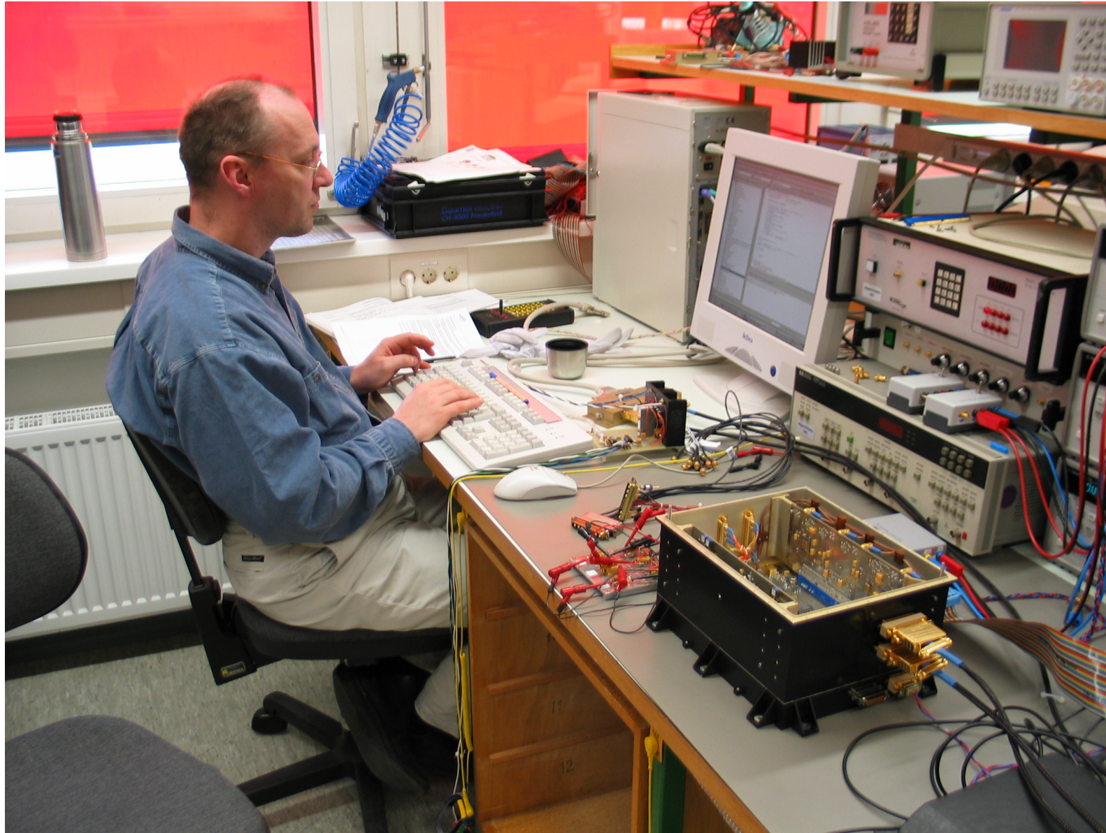
Functional testing of the WBS electronic box at the MPS in the microwave laboratory (R-Building).
