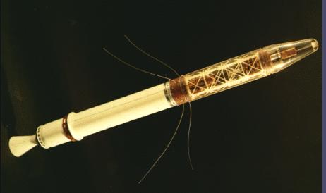
Explorer 1 (Jan 31, 1958) carried a Geiger Counter to study the latitudinal distribution of low-energy cosmic rays. It failed miserably in that
