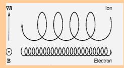
The ratio in front of the gradient term is the particle's **magnetic moment**, i.e. the ratio between the kinetic energy and the magnetic field:
