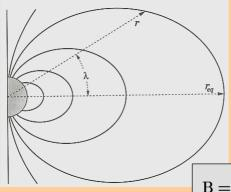
At distances not too far from the surface the Earth's magnetic field can be approximated by an azimuthally symmetric *dipole field* with a moment:
