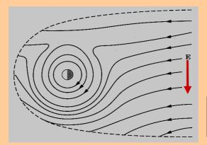
Solar wind generates an electric field from dawn to dusk in the equatorial plane. Particles will *drift sunward* in this field.
