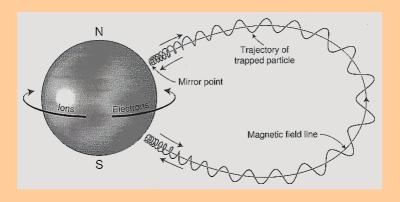
A *dipole magnetic field* has a field strength minumum at the equator and converging field lines at the polar regions (mirrors). Particles can be *trapped* in such a field. *They perform gyro, bounce and drift motions*.
