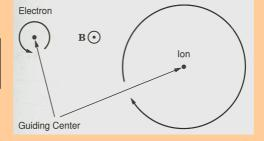
The equation describes a circular orbit around the field with gyroradius,  $r_g$ , and gyrofrequency,  $\omega_g$ . The orbit's center  $(x_0, y_0)$  is called the **guiding center**. The gyration represents a microcurrent, which creates a field opposite to the background one. This behaviour is called **diamagnetic effect**.
